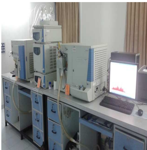
LC-MS/MS: Liquid Chromatography with Mass spectrometer(Ion Trap & Triple Quadruple)
