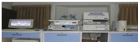
HPLC: High Performance Liquid Chromatography
