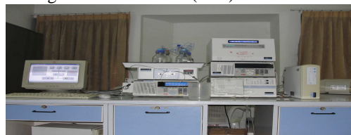
HPLC: Quaternary gradient system. Variable operating back pressure 5000psi, Detectors: Photo Diode Array(PDA),UV-VIS, Fluorescence Detector
