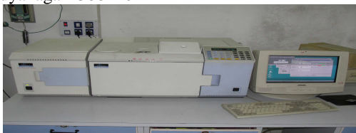
GC-MS: Analyser: Single Quadrupole with Prefilter, Mass range: 20-650 Daltans (amu).
