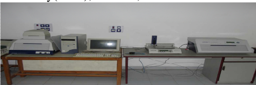
HPTLC: Automatic applicator (Linomat-5), scanner-3 and documentation (reproster-3).Scan range :(190nm to 800nm)
